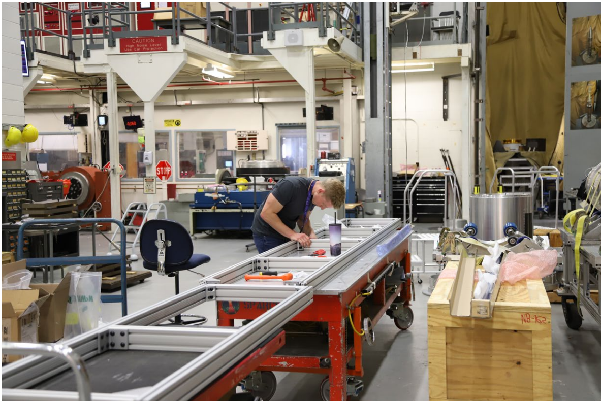
Construction of a new horizontal deployment fixture in the Testing and Evaluation Lab. Credit: NASA Photo/Berit Bland
